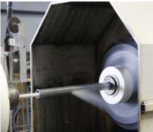
Fiber Reinforcement Wrapping
