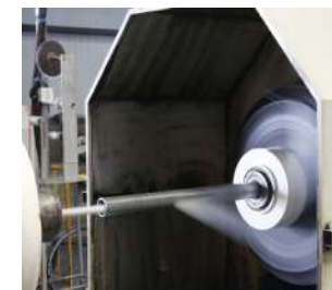
Fiber Reinforcement Wrapping
