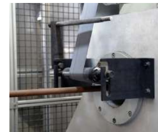
Fiber Reinforcement Wrapping
